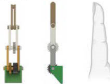
Figure 1. Design Prototype. Mechanical components (gears and conveyor belts) are aligned with finger joints.
