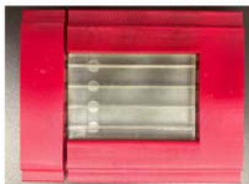
Figure 2: Early stage physical prototype of microfluidic chip holding device: This prototype was 3D printed and includes a sample resin printed microfluidic chip.
