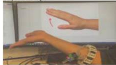
Figure 2. An example of using Optoband and graphical user interface application developed for hand gesture recognition.
