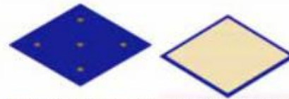
Figure 1: Pad, deconstructed as two layers (black squares represent hydrosensors, white part is absorbent layer).
