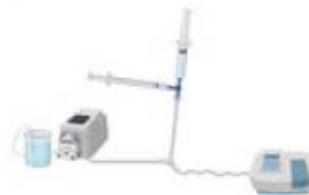
Figure 2. Customized testing apparatus for UV-Vis kinetics studies.
