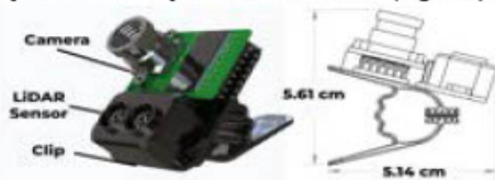
Figure 1. EchoAware clip-on LiDAR sensor and camera
